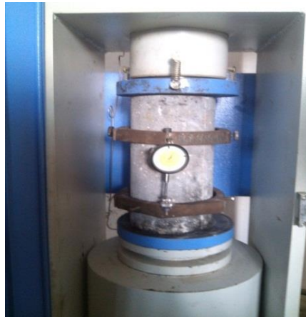
Fig: specimen set up to find stress strain behavior
